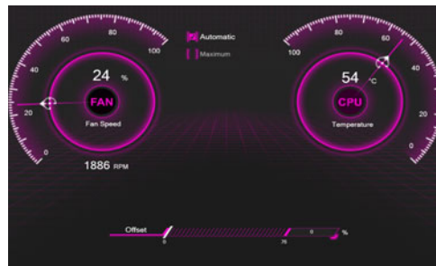
Figure 9 - Fan Speed Control
